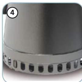
Strainer A special set allows the sewage pump to be transformed into a dry floor one. The minimum level of liquid can be lowered to 5 mm from the ground by setting two special shimming.
